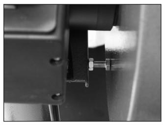
**Figure 11.** Adjusting collector support plate bolts.
